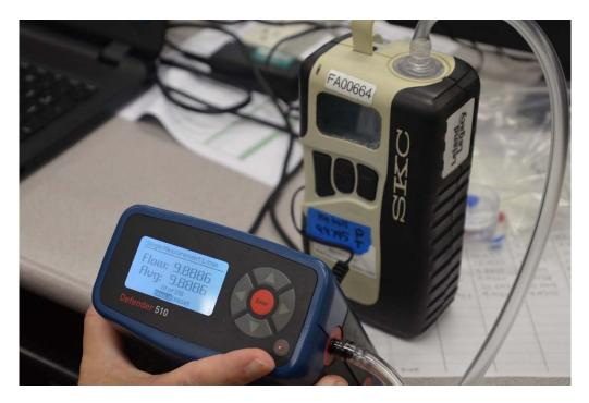
Photo 1 – Equipment calibration with a direct read primary standard traceable to NIST<sup>1</sup>
